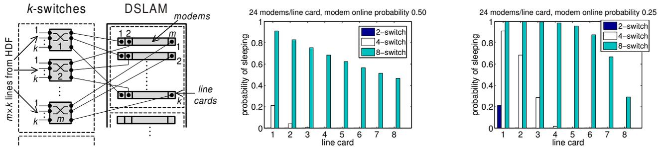
Figure 5: [left]  $k$ -switches and connection to DSLAM. [middle and right] Probability of line card 1, 2, ...,  $k$  sleeping on a batch of  $k$  line cards connected through  $m$   $k$ -switches. Each line card has  $m = 24$  modems and each modem is active with probability  $p = 0.5$  (middle) or  $p = 0.25$  (right).
